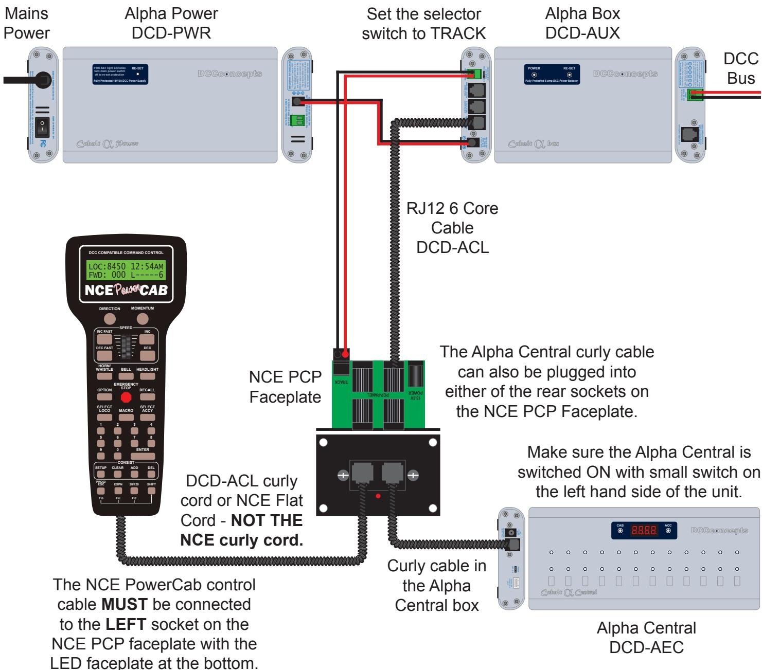
The NCE PowerCab control cable **MUST** be connected to the **LEFT** socket on the NCE PCP faceplate with the LED faceplate at the bottom.
