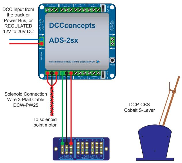
To reverse the output wires to match the lever throw, swap the green and red wires at the relevant Cobalt S-Lever or ADS connection.
