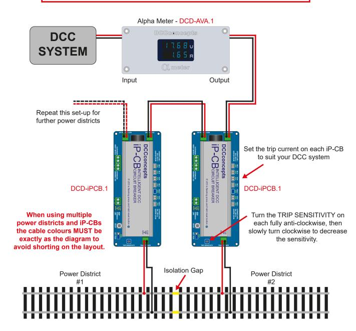
If a short occurs between two power districts on the layout, swap the output wires from the iP-CB that is connected to that power district.
