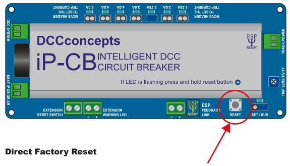
The iP-CB can be reset to factory settings without using the CVs by using the following process:
