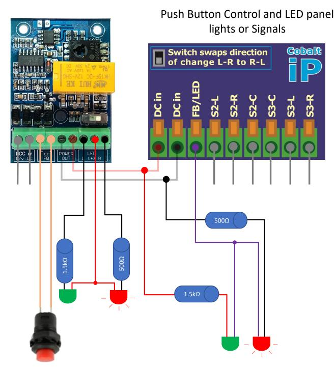
Push Button Switch toggles the turnout L > R > L (etc)
