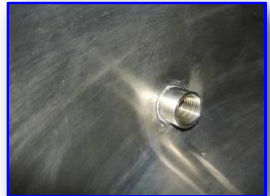
Stainless sheet with a piece of stainless tube soldered into it
